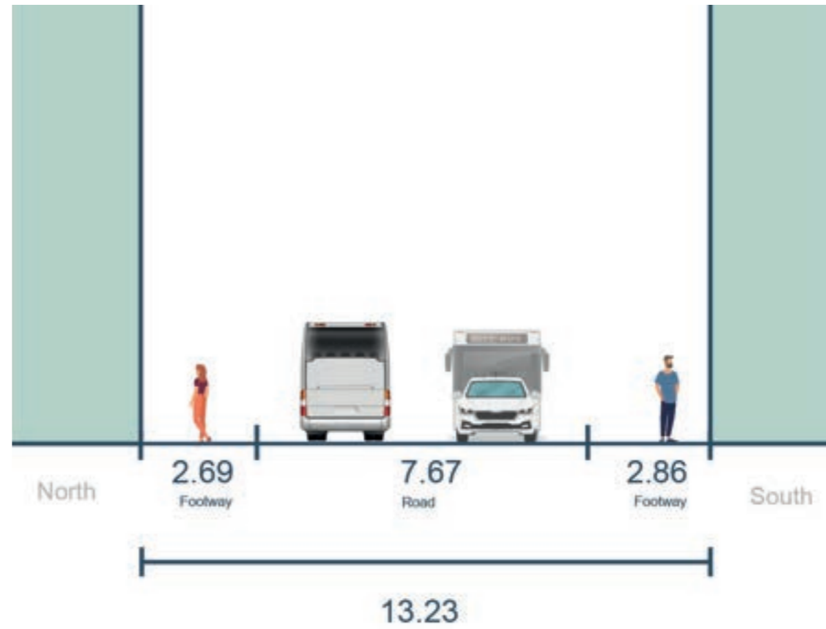
Figure 56 - Existing street section
