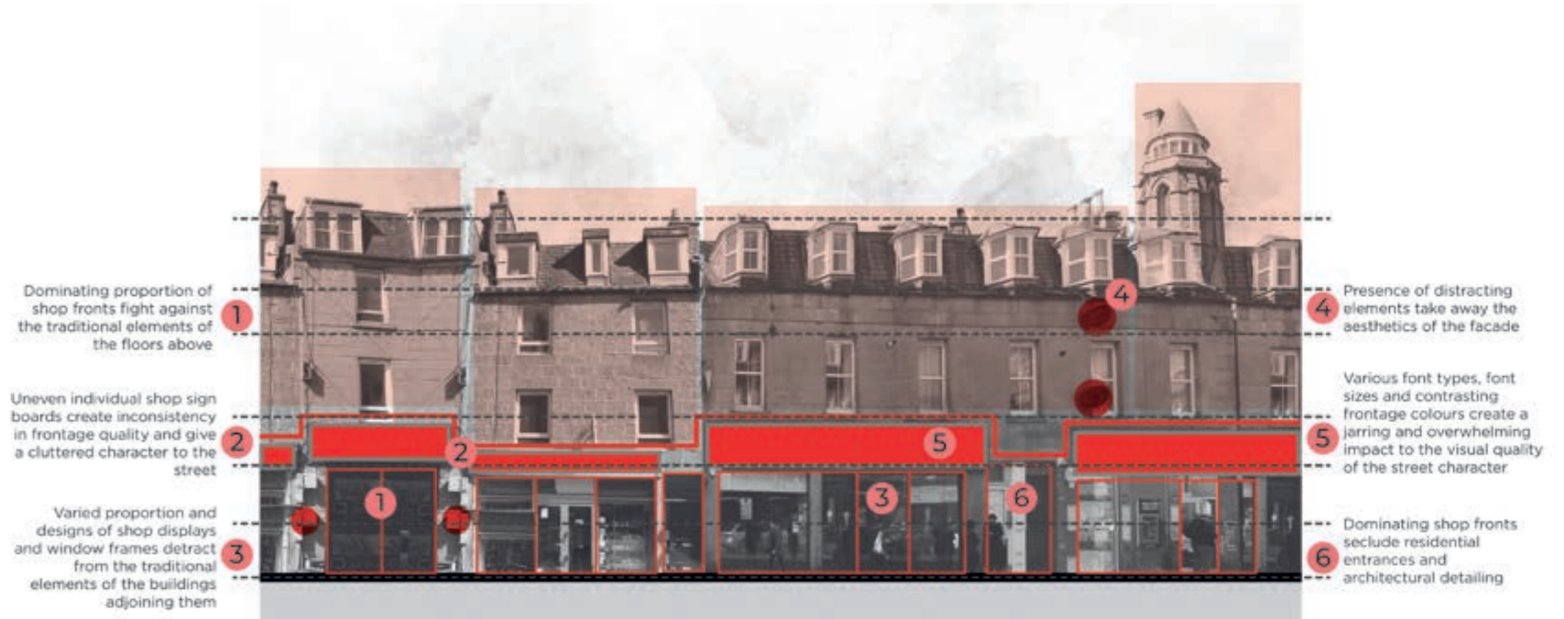
Inconsistencies in George Street's shop frontage
