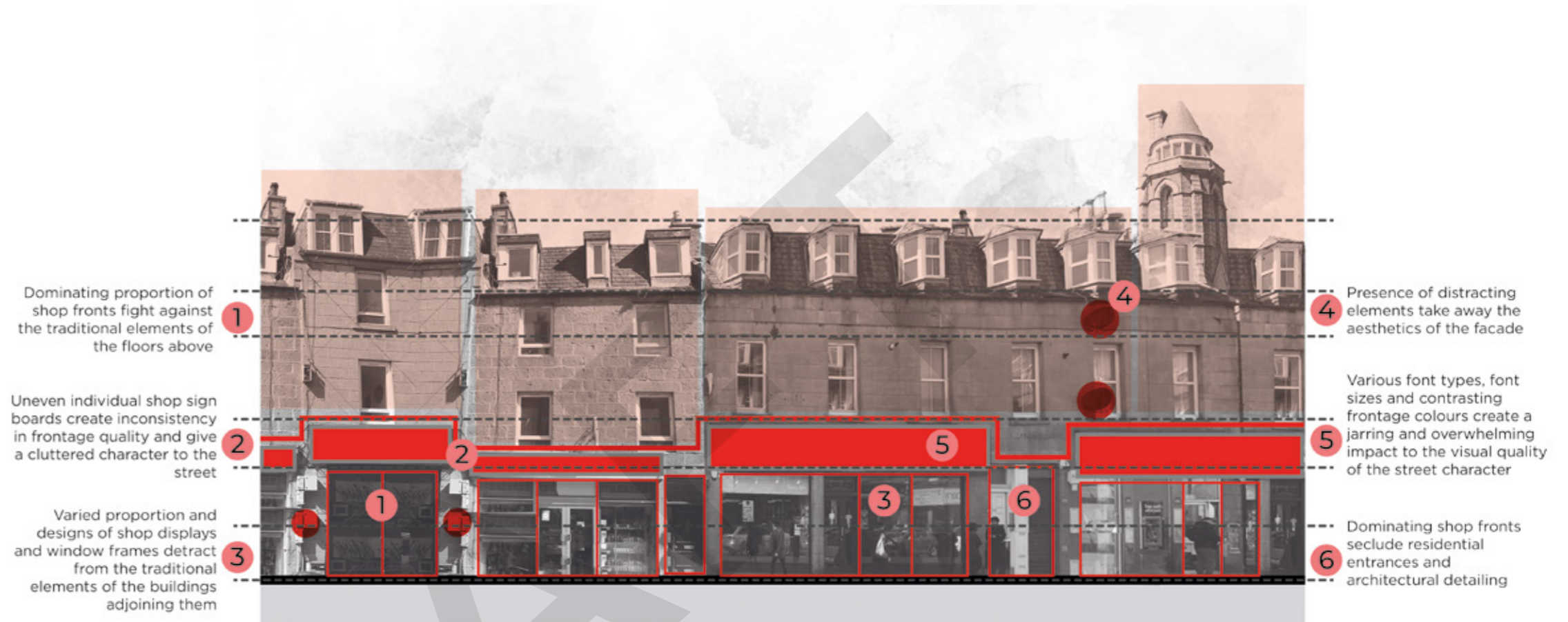
Figure 30 - Inconsistencies in George Street's shop frontage
