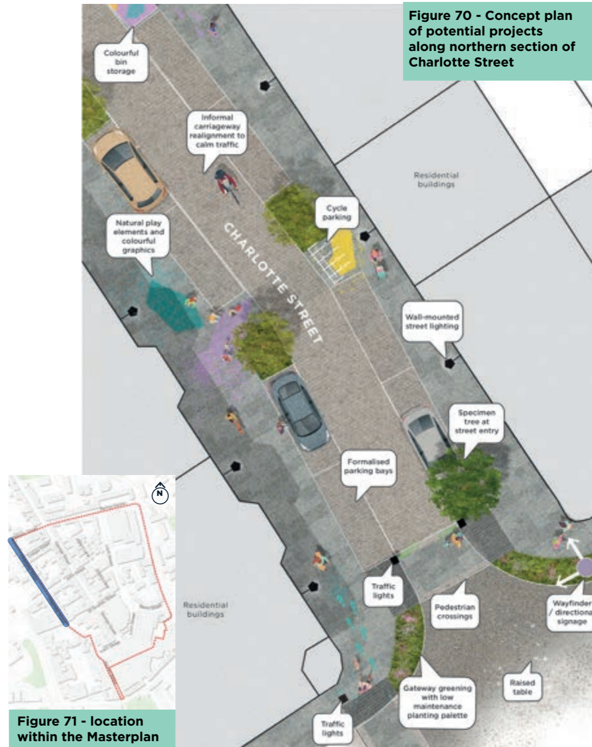
Subtle road alignments can help manage traffic speeds in residential areas
